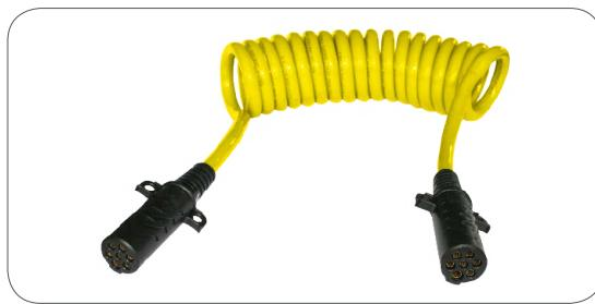
7P/12V EXPERTECH™ coil with DURACORE™ plugs - SAE J560 Auxiliary yellow cable (4x 3.0mm<sup>2</sup> + 2x 5.0mm<sup>2</sup> + 1x 8.0mm<sup>2</sup>), coil diameter: 100mm
